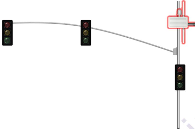
**Figure 14: An example illustration of RSU-352 mounting on a vertical mast/post**
