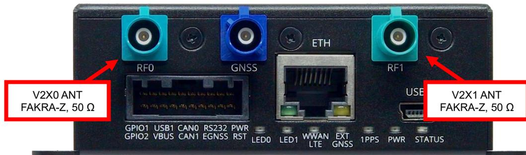
**Figure 10: V2X antenna ports**
