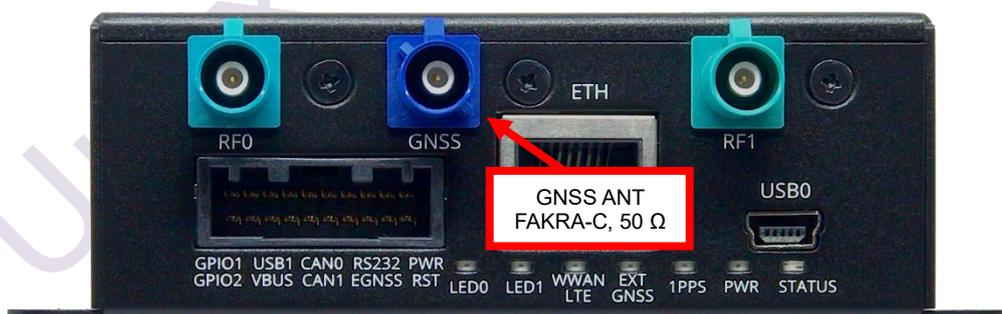
**Figure 11: GNSS antenna port**
