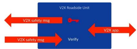
Security functions provided by V2Xcast<sup>®</sup> are designed based on a highly secure HSM (Hardware Security Module).
