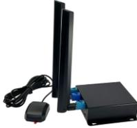
As an external V2X modem: connect V2X OBU to vehicle's existing application ECU through Ethernet and develop the application software
