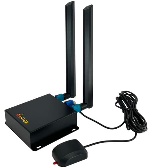
OBU-352 is the most advanced V2X on-board unit featuring a global V2X solution; the hardware supports either C-V2X or DSRC-V2X communication standards with appropriate V2X stack embedded, reducing the cost and complexity for global deployments.
